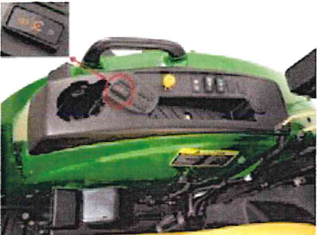
Optional cruise control on 4M Tractors
