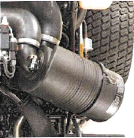
Air filter with air-restriction indicator
