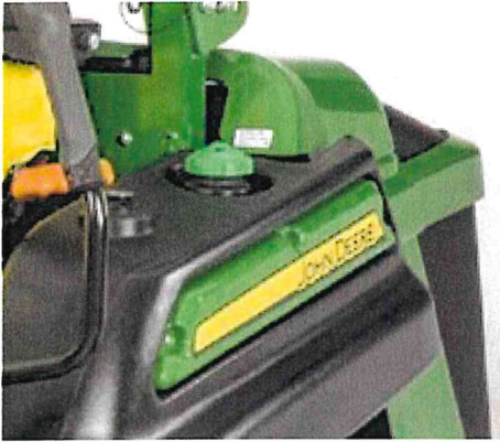
Fuel tank and fuel gauge
