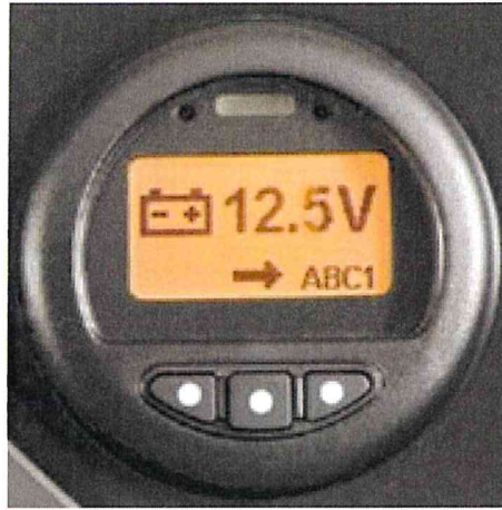
System voltage screen
