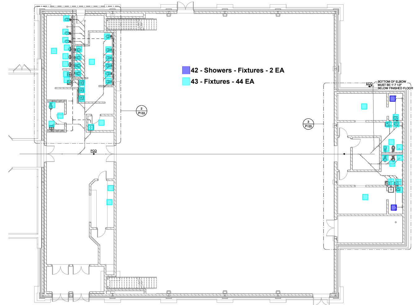
1 BELOW FLOOR PLUMBING PLAN - GYMNASIUM ADDITION 1/8" = 1'-0"
