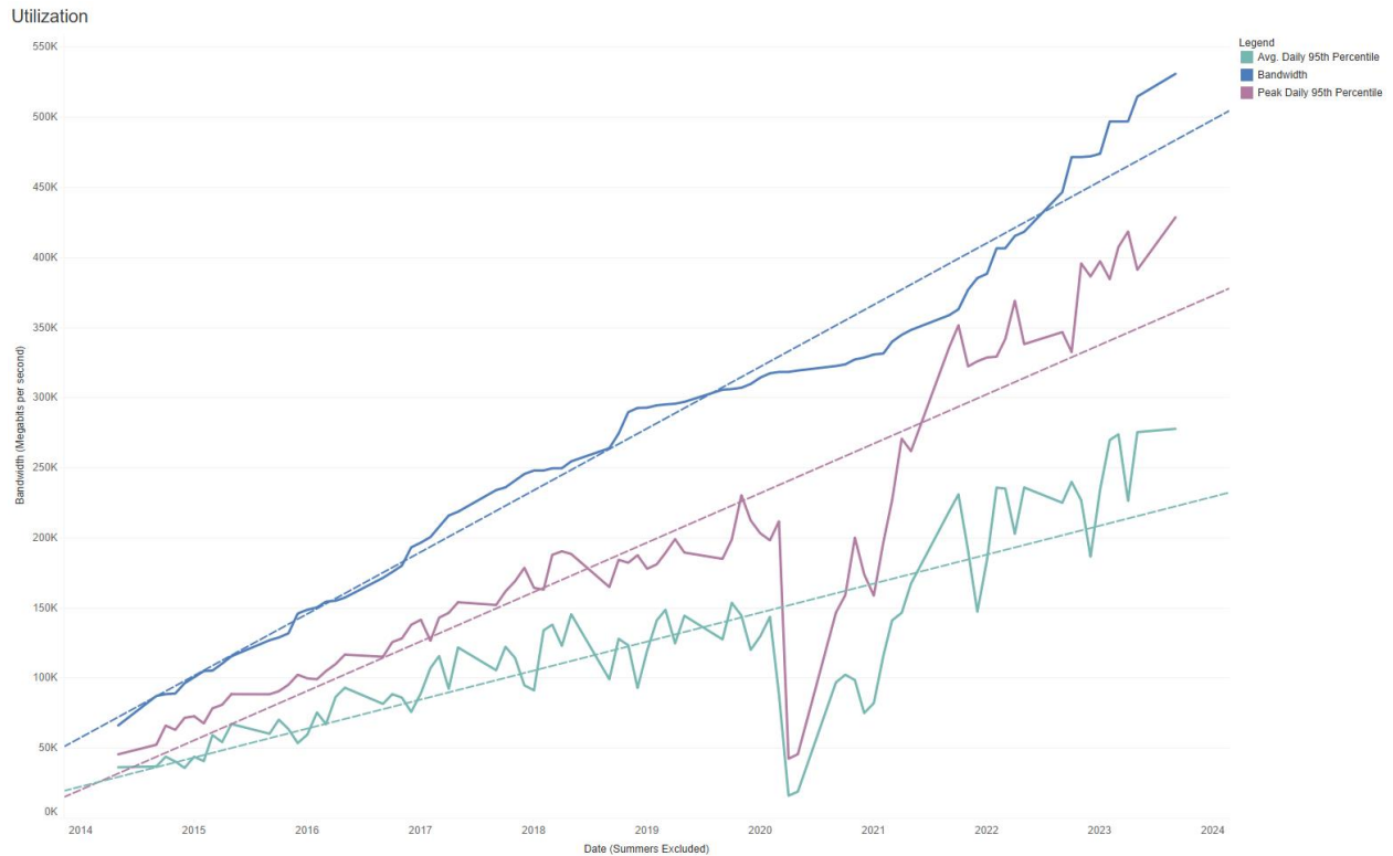
Figure 3: Statewide Contracted Bandwidth, Peak, and Average Utilization for all PSUs using NCREN.
