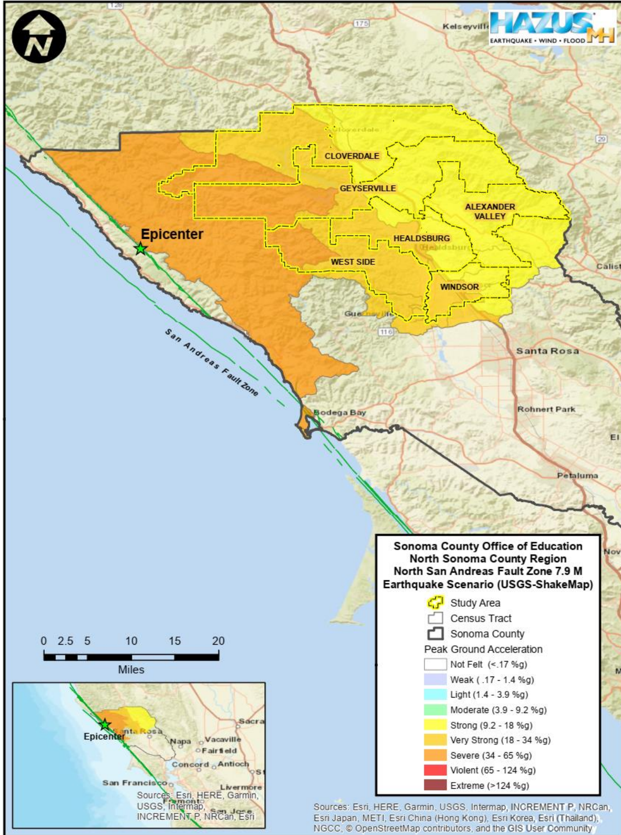
Map: Shake Intensity Map – San Andreas Fault M7.9 – North Sonoma County Region (Source: Emergency Planning Consultants)
