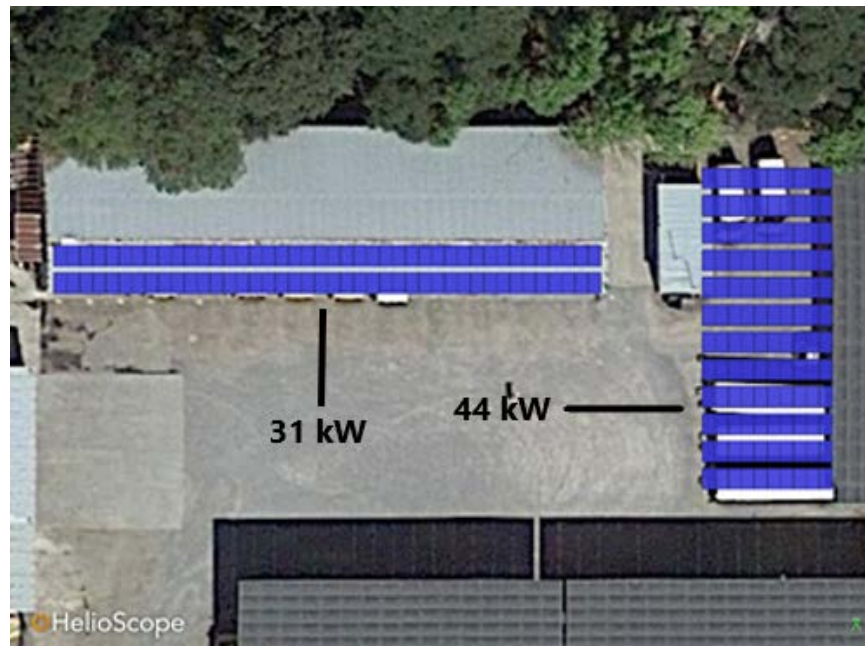
Figure 17. Analy High School Additional Solar Technical Feasibility
